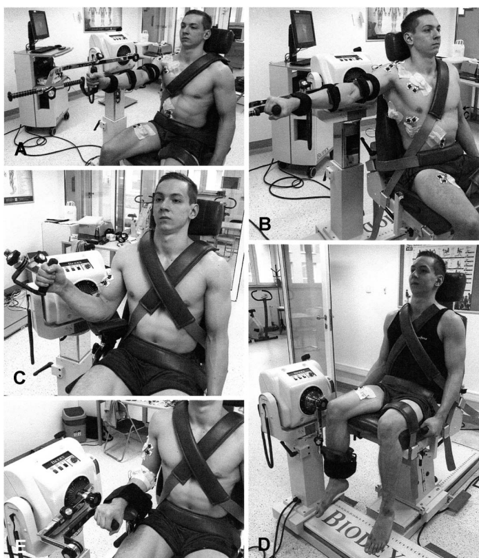
Figure 1. The setup and positions of gymnasts during recording of a maximal voluntary contraction at arbitrary angles that were used for electromyographic normalization. A) Shoulder joint (sagittal plane)—anterior deltoid (flexion), pectoralis major, and the latissimus dorsi (extension); B) shoulder joint (frontal plane)—trapezius descendens and the lateral deltoid muscles (abduction); C) elbow joint—biceps and the triceps brachii (flexion and extension, respectively); D) knee joint—rectus femoris (extension); E) wrist joint—wrist flexors and extensors.
